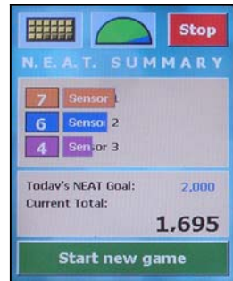
Fig. 7. Graphing bars show activity of 3 wearable motion sensors in real-time
