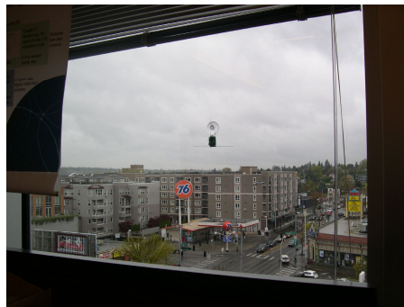
Fig. 6. WISP mounted by suction cup to interior window for light level measurement experiment
